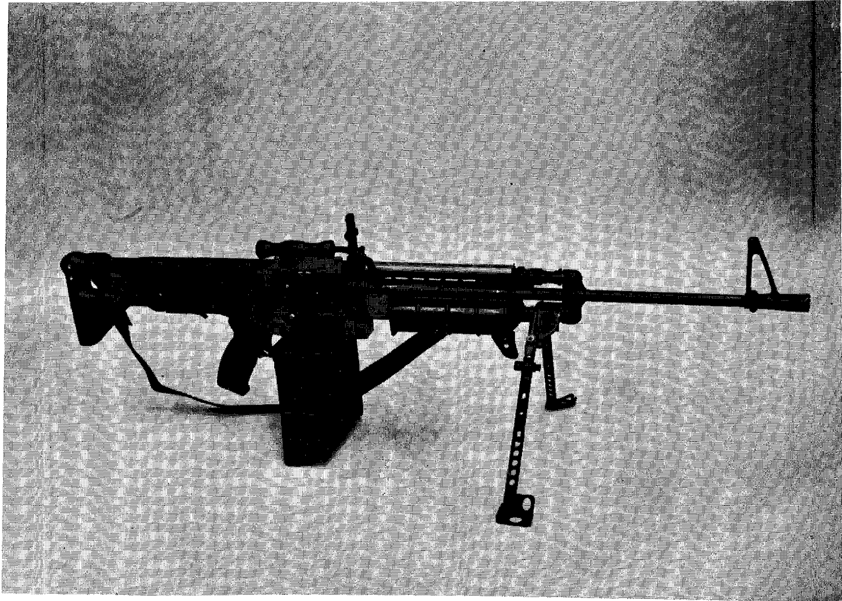
XM248 Weapon with 200-Round Magazine. Bipod erect with legs retracted.
