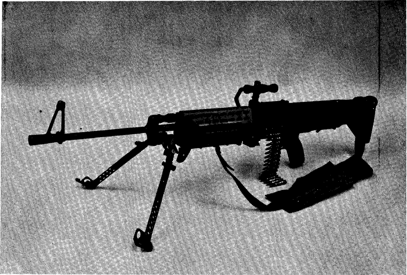
Figure 1-1. XM248 weapon with free hanging belt. Bipod set low in forward cant position.
